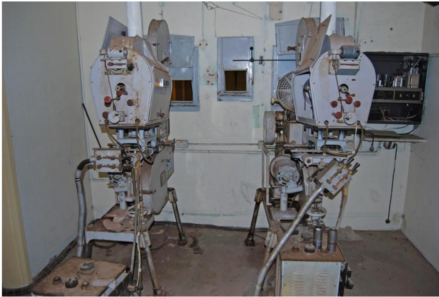
The original carbon arc projectors in situ in the first floor projection room
