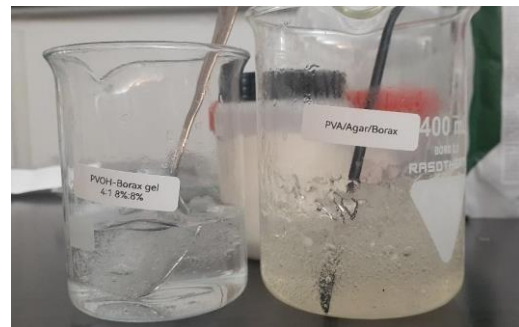
Figure 6 Final appearance of hydrogels such as Borax gel and mixture of PVA/Agar/Borax. (Photo courtesy: H. Tandy)
