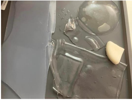
Figure 7 Final appearance of hydrogels such as Agar-Agar, Gellan gum, pure Borax, and Konjac. (Photo courtesy: H. Tandy)
